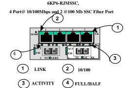
module of the 6K16-Series Switch supporting four Copper and two single-mode fiber network segments.
